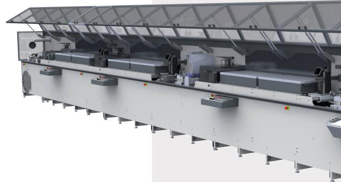
The **Solar** is the result of years of experience with OPV solar coating machinery. It is an R&D machine with industrial output capacity. With this machine your research team can get the best of two worlds and experiment with future coatings. The machine is designed to work with organic, perovskite and other related PV technologies, OLED, LEC and many more.
