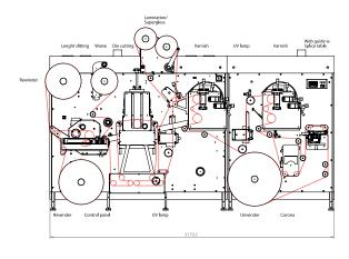
DC330HYBRID finishing line. Hybrid laser and traditional die cutting. Flexo varnish with spot, lamination, coldfoiling, semi-rotary die cutting, slitting and dual rewind.
