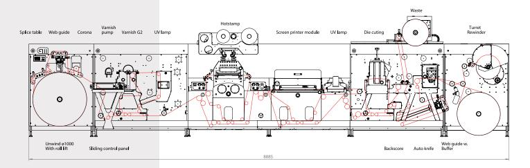
DC350 finishing line with combined 50-ton high quality flatbed hot foil stamping and flatbed screen printing. In addition semirotary GM SmartFlexo, semi-rotary die cutting, GM SmartStrip, GM SmartSlit and GM SmartTurret - NEW fully servo controlled automatic turret rewinder.
