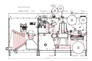
DC330MINI finishing line with inline option for HP Indigo digital press. This configuration offers compact and economic processing of labels. Features: flexo varnish, lamination, spot varnish and semi-rotary die cutting.
