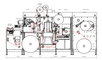
DC330MINIflex finishing line with the powerful smart essential options. Compact and economic processing of labels with flexo varnish, lamination, spot varnish, semi-rotary die cutting, autoslitting and semi automatic turret rewinder
