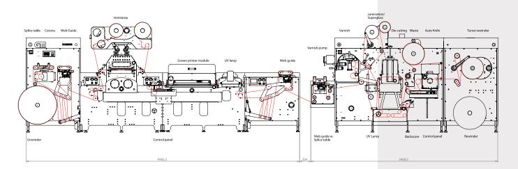
**330FB** Premium Wine Label Finisher inline with **DC330MINIflex**. High quality 50-ton flatbed foil stamping and flatbed screen printing with servo register and foil saver. Embossing and hot foiling can be done using the same tool. DC330MINIflex expands the finishing potential with flexo varnish, lamination, spot varnish, semirotary die cutting, autoslitting and rewinding on semi automatic turret rewinder.
