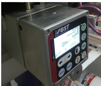
As standard the unit features a BST web guide with an ultra-sonic fork. The web guide supports normal and transparent webs.
