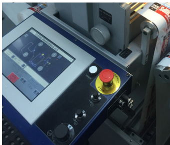
Large 10" color touch display with clear indication of web path. Knobs for stepless tension setting on rewind spindles.
