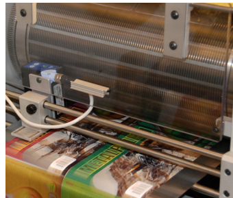
High precision servo controlled semi-rotary die cutter. Perfect re-register to digitally printed webs. Support for marks on transparent web.
