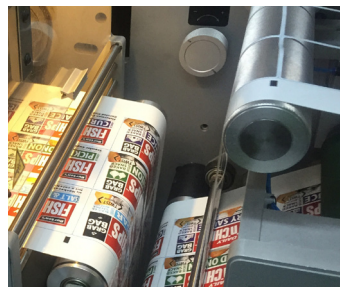
Matrix stripping at a breeze. Two roller design - first a strip roller with anti-stick coating and then a waste rewind. Both with stepless tension.
