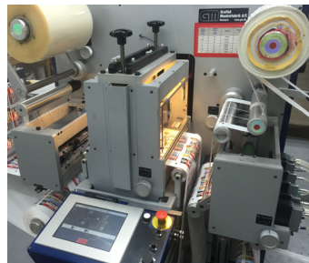
The short distance from unwind to rewind ensures minimum waste of material. The machine is easy to web up due to cantilevered design.
