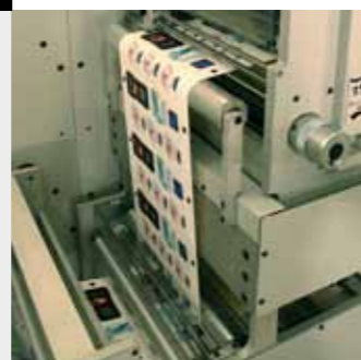
Heavy die cutter: Heavy semi-rotary die cutter for 330 and 500 mm web.
