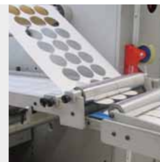
Conveyor: Drop-in conveyor for sheet or free-shape production runs.
