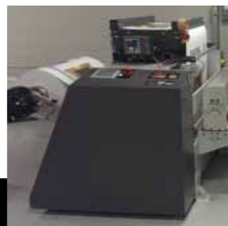
Jumbo unwinder with hydraulic lift from floor.
