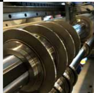
Automatic knife box. Set all knives in 30 seconds.
