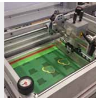
Flat bed screen unit with pneumatic frame lock.
